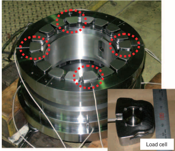
図10 スラスト力測定用軸受 Fig.10 Thrust bearing with load cell (for measurement of gas thrust force)
