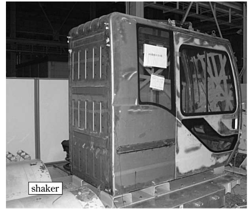
図12 加振試験 Fig.12 Shaker testing of cabin
