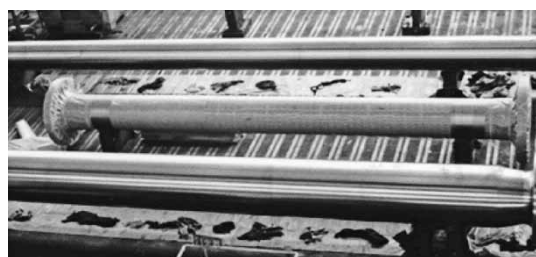
図2 中間軸の外観 (機械加工後) Fig. 2 Appearance of intermediate shaft after machining
