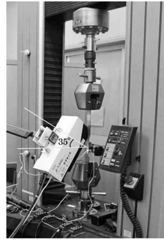
図2 X線応力測定の精度確認用引張試験 Fig.2 Tensile test to confirm accuracy of X-ray stress measurement
